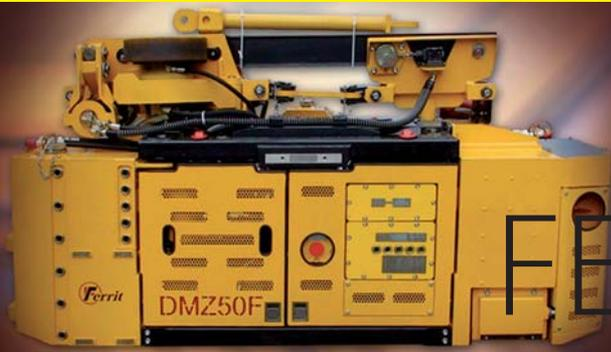
SUSPENDED MINING MANIPULATOR DMZ50F
