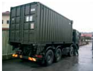
20' ISO 1C Transport container NSN code 8145-42-0000052 Loading the container on a vehicle (ROLLBAR Loading System)
