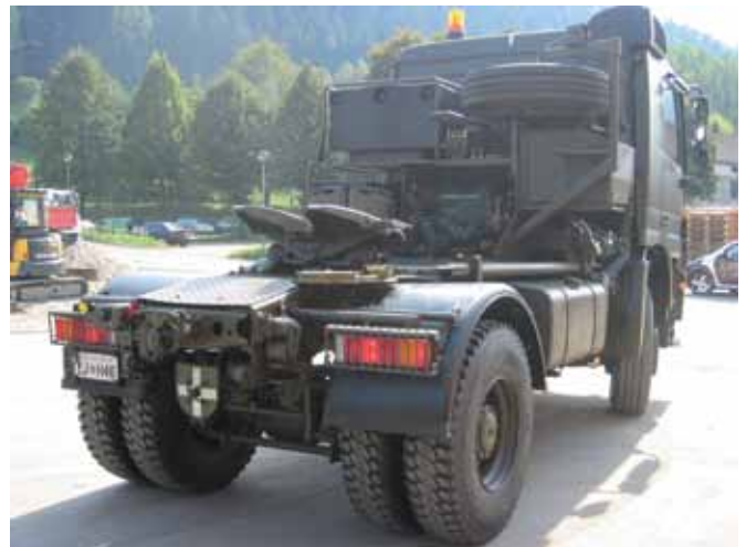
Recovery vehicle with two winches and three-wheel coupling
