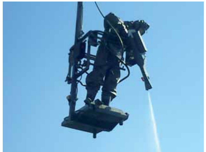
Working basket with Kärcher Decontamination system
