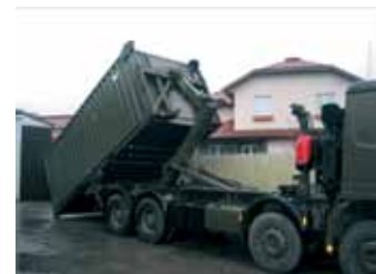
20' ISO 1C Transport container NSN code 8145-42-0000052 Loading the container on a vehicle (ROLLBAR Loading System)
