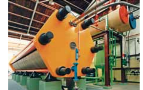
Electrolyser producing hydrogen from windpower
