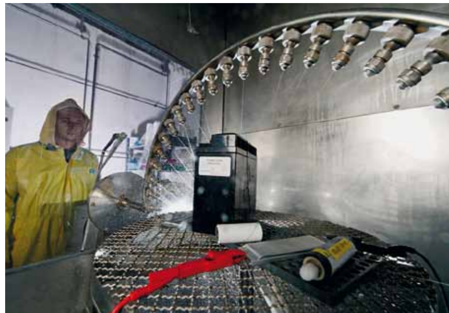
Simulation of environmental conditions (rain water test) which forms part of our development of concepts to ensure safety. It includes testing of batteries subjected to malpractice.
