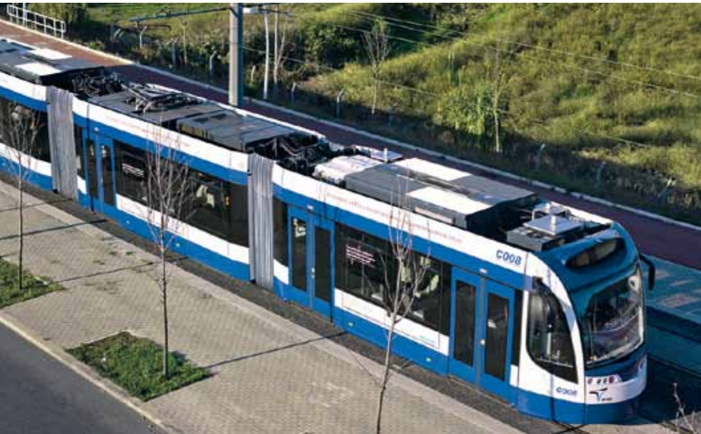
Fitted with a hybrid energy storage system (Siemens) street cars can cover up to 2,5 km without overhead power connections. This is made possible by employing a combination of electric double-layer capacitors (EDLC) and a nickel-metal-hydride battery. These enable the braking energy to be stored effectively and utilized for supporting the traction. This has a number of benefits such as: power consumption is reduced by a third, thereby cutting emissions by 80 t CO 2 p.a.; power cables can be removed from areas where they are a visual blight (e.g. in historical malls) or where it is inconvenient to keep and maintain them (e.g. at traffic intersections or in tunnels).
