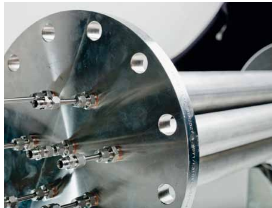
Europe's largest hydrogen storage tank based on complex hydrides and containing 8 kg of sodium alanate storage material, constructed and built at GKSS
