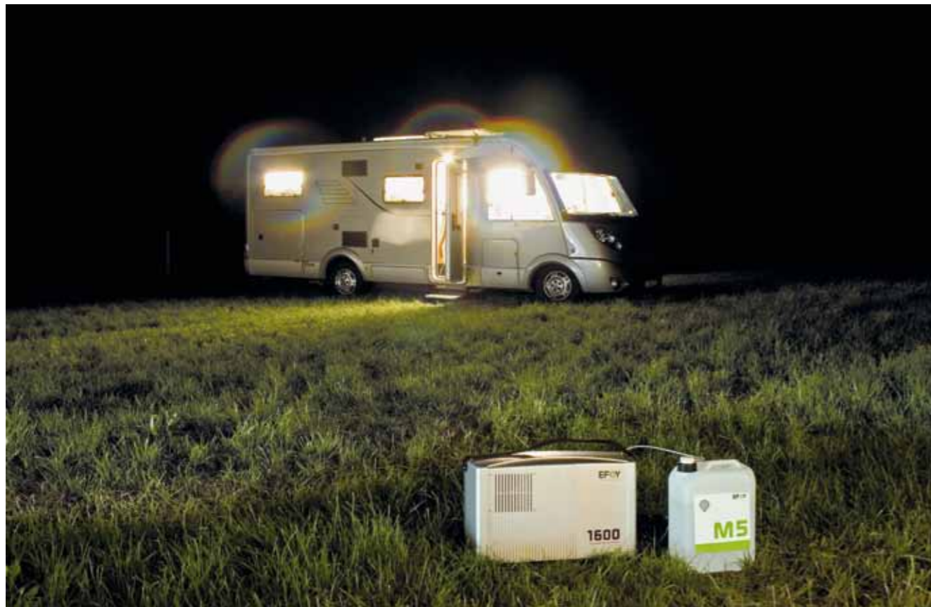
Fuel cells used for auxiliary power supply of mobile and portable applications (up to 250 W) are under development. The use of fuel cells to provide stand-alone power in mobile homes, sailing boats, holiday cottages and hunting and hiking lodges is well established.
