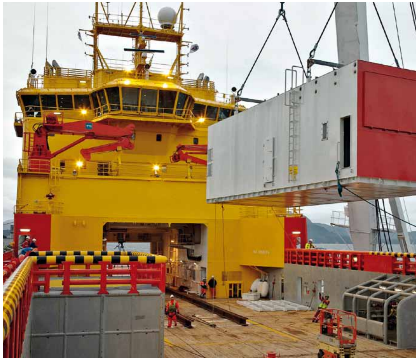
The container with the HotModule for the Viking Lady is transported to be performance tested. The fuel cell stack is integrated into a rectangular metal container.
