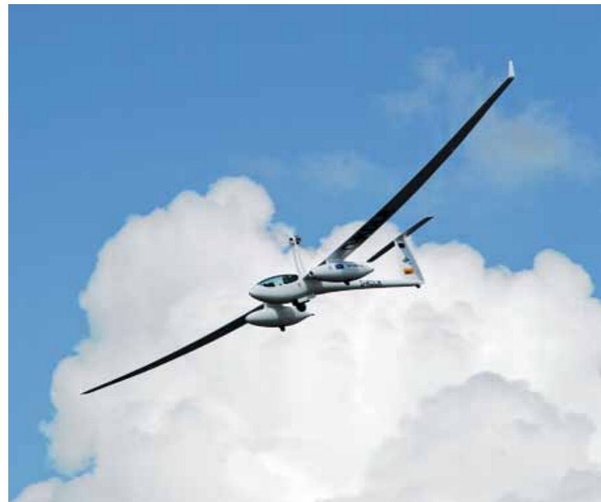
In 2009 the first airplane (Antares DLR-H2) powered by fuel cells lifted off from Hamburg airport. The use of fuel cells has the following benefits: The exhaust is totally free of particles and consists only of water. If hydrogen is produced by renewable energies, the plane is powered without generating any CO 2 .
