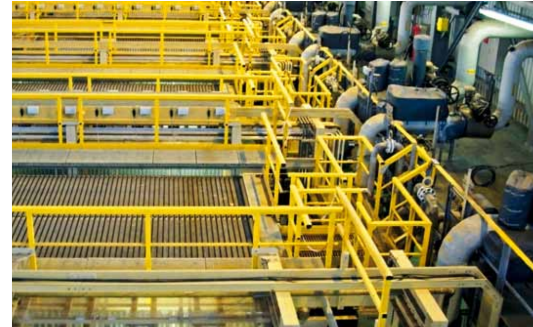
Membrane electrolysis producing chlorine: Dow Chemicals in Stade. Power consumption: 600 MW, hydrogen is generated as a co-product.
